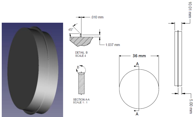
Figure 30: Geometry used for ECHO3D simulation of the ESR flange weld step.
