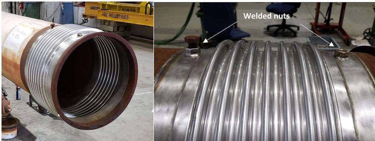
Figure 1 Bellow nut restraint installation
