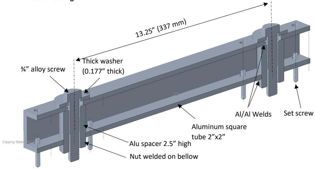
Figure 2 CAD model of the restraint design
