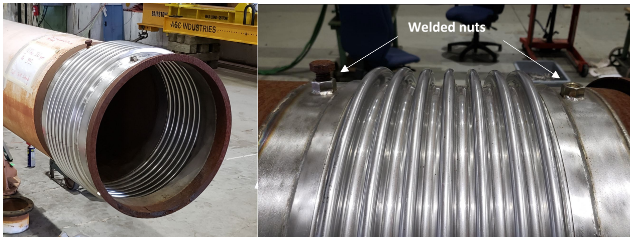
Figure 1 Bellow nut restraint installation
