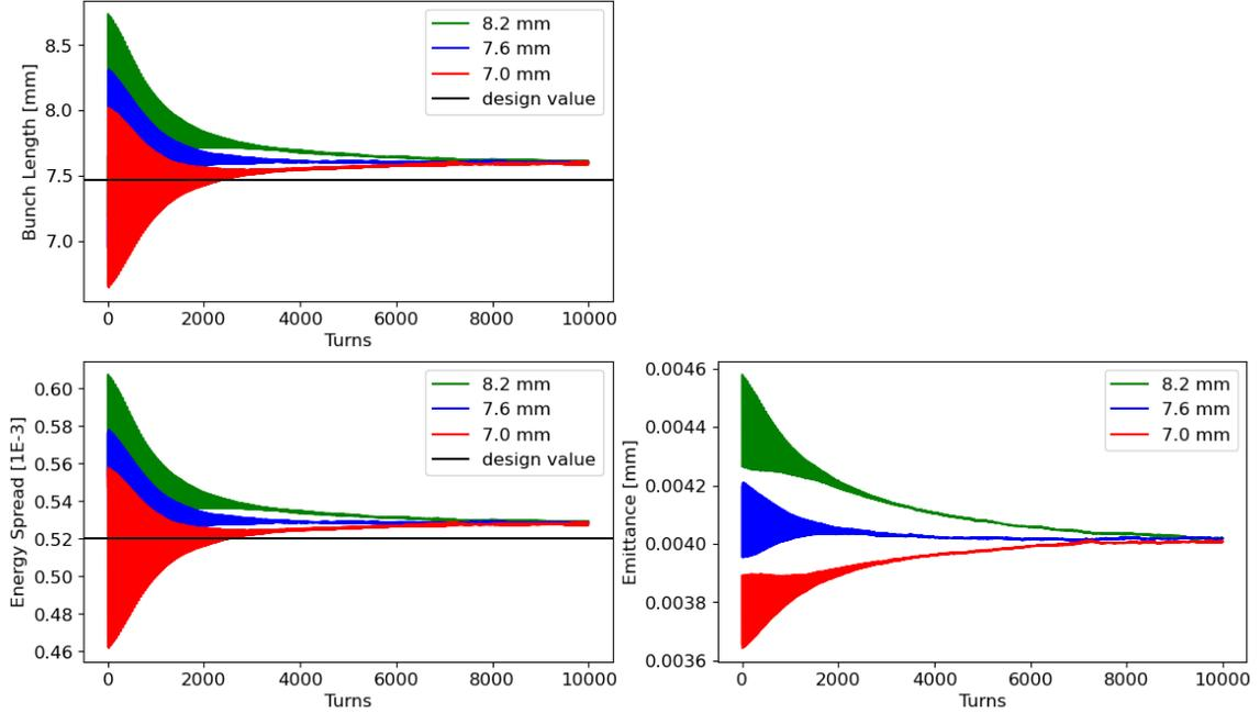
**Fig. 4:** The plot illustrates the bunch length (top), energy spread (bottom left), and longitudinal emittance (bottom right) as a function of tracking turns for three different initial beam sizes 7.0mm, 7.6mm and 8.2mm, while the energy spread is kept same.
