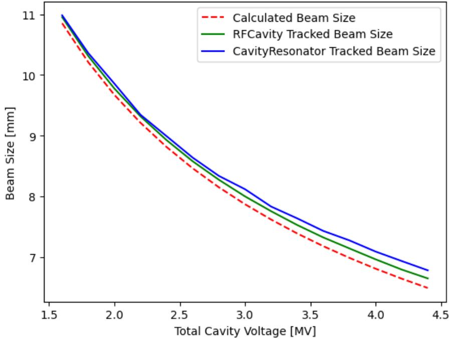
**Fig. 5:** The plot depicts the relationship between the bunch length and RF cavity voltage for two methods: the RFCavity method (represented by the green curve) and the CavityResonator method (represented by the blue curve). The corresponding theoretical results for each method are shown as dashed lines.
