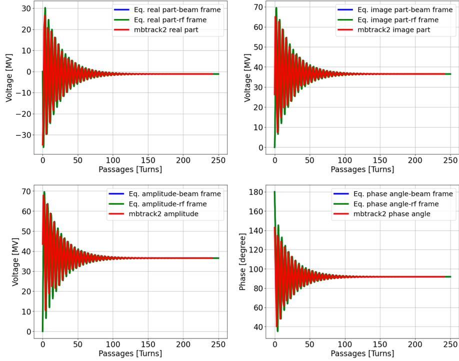
**Fig. 7:** The plot shows the beam-induced voltage calculated with formula in beam-frame and RF-frame, as well as from the Mbtrack2 tracking.
