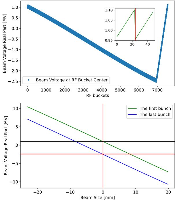
**Fig. 8:** The top plot shows the beam induced-voltage as function of the bunch train or RF buckets. The bottom plot shows the beam-induced voltage as function of longitudinal macroparticle position in a bunch.
