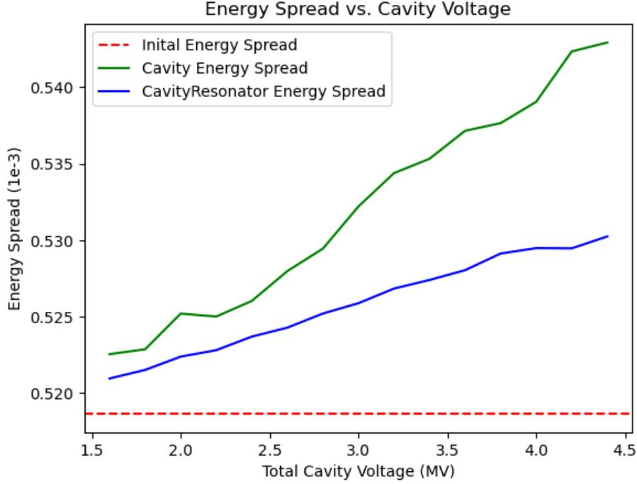
**Fig. 6:** The plot depicts the relationship between the energy spread and RF cavity voltage for two methods: the RF cavity method (represented by the green curve) and the Cavity Resonator method (represented by the blue curve). The corresponding theoretical results for each method are shown as dashed lines.
