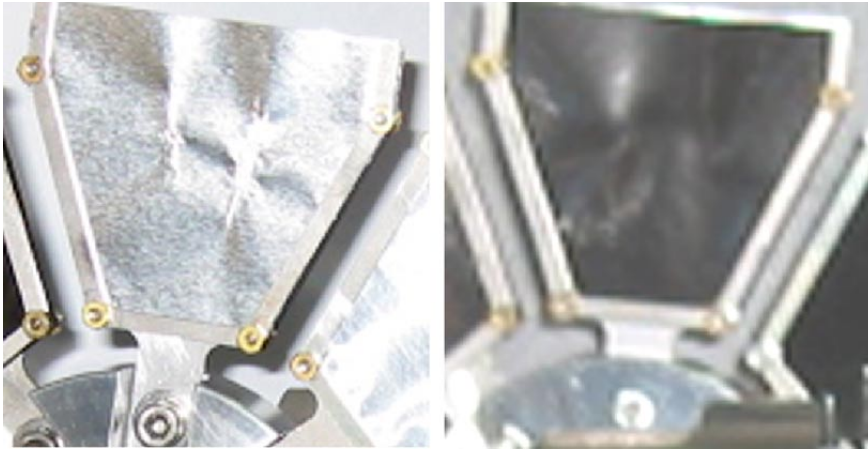
Figure 3.3: Deformation of the Al-C foil as documented in [13].
