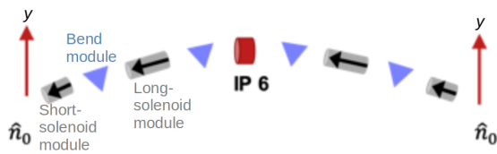
Figure 3: The spin rotators are composed of short- and long-solenoid modules, as well as bend modules, to rotate the spin from vertical in the arcs to longitudinal at the IP and back to vertical on the other side.
