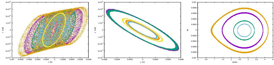
Figure 18: Monitoring: 185,000-turn phase spaces, a few particles (different colors), observation is at 9 o'clock snake. Horizontal oscillation of  $\pm 1 \text{ mm}$  (left graph) is for  $dp/p \approx 10^{-3}$  excursion (right) hence a local dispersion at 9 o'clock snake of about 1 m.
