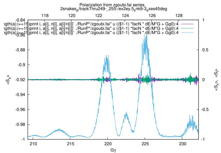
Figure 11: Crossing 249-Qy and 255-Qy, proton, 2 snakes, collision optics,  $\epsilon_x/\pi = \epsilon_y/\pi = 2.5 \mu\text{m}$ , Closed orbit is zero. Turn-by-turn  $\langle S_y \rangle$  (left axis), and  $\langle S_l \rangle \langle S_x \rangle$  (right axis),  $\hat{V} = 35 \text{ kV}$ ,  $10^6$  turns.
