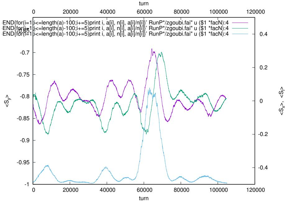
Figure 22: Proton,  $\epsilon_x/\pi = 2 \mu\text{m}$ ,  $\epsilon_y/\pi = 0.5 \mu\text{m}$ , case of 0.61 mm rms vertical defect orbit. Just 1 seed. Turn-by-turn  $\langle S_y \rangle$  (left axis), and  $\langle S_l \rangle$   $\langle S_x \rangle$  (right axis) 1,000-particle averages. Polarization difference in start and end regions is < 1%.
