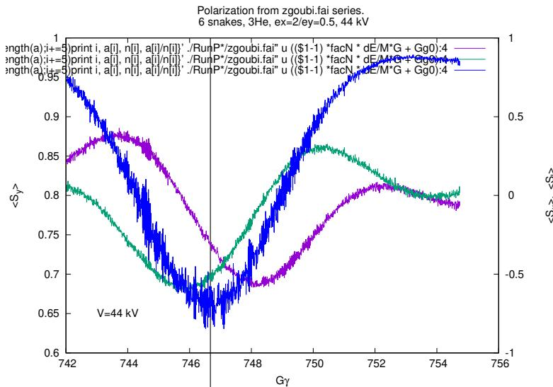
Figure 42: 3He, 6 snakes,  $\epsilon_x/\pi = 2 \mu\text{m}$ ,  $\epsilon_y/\pi = 0.5 \mu\text{m}$ . case of 0.61 mm rms vertical defect orbit. Turn-by-turn  $\langle S_y \rangle$ , and theoretical envelop (left axis), and  $\langle S_l \rangle$   $\langle S_x \rangle$  (right axis) 500-particle averages,  $\hat{V} = 44 \text{ kV}$ .
