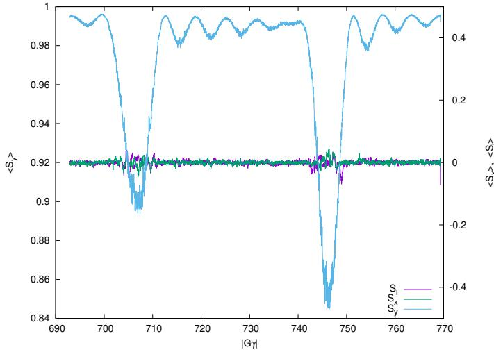
Figure 39: Turn-by-turn  $\langle S_y \rangle$ ,  $\langle S_l \rangle$  and  $\langle S_x \rangle$  1,000 particle averages across  $735-\nu_y$  and  $717+\nu_y$ , helion.  $\nu_y = 29.6730$ .  $\epsilon_x/\pi = \epsilon_y/\pi = 2.5 \mu\text{m}$  normalized.  $\hat{V} = 300 \text{ kV}$ ,  $\phi_s = 2.7925$ ,  $\dot{\gamma} = 6/\text{s}$
