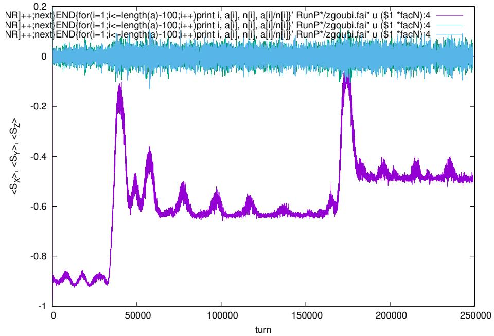
Figure 29: Helion, turn-by-turn  $\langle S_y \rangle$ ,  $\langle S_l \rangle$  and  $\langle S_x \rangle$  1,000 particle averages across  $735-\nu_y$  and  $717+\nu_y$ , helion,  $\epsilon_x/\pi = \epsilon_y/\pi = 2.5 \mu\text{m}$  normalized.  $\hat{V} = 300 \text{ kV}$  ( $\dot{\gamma} = 6$ ), no need to check 35 kV.
