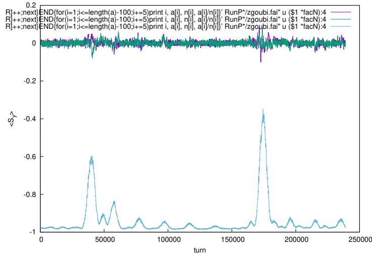
Figure 31: Turn-by-turn  $\langle S_y \rangle$ ,  $\langle S_l \rangle$  and  $\langle S_x \rangle$  1,000 particle averages across  $735-\nu_y$  and  $717+\nu_y$ , helion,  $\epsilon_x/\pi = 2 \mu\text{m}$ ,  $\epsilon_y/\pi = 0.5 \mu\text{m}$  normalized.
