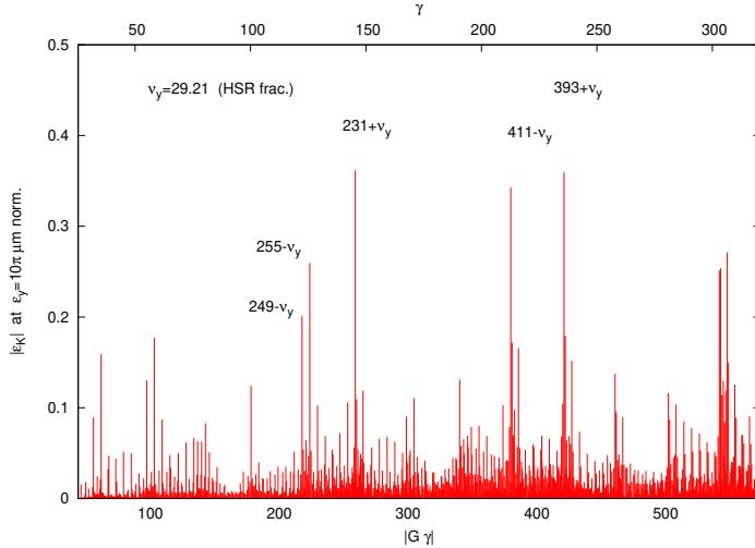
Figure 4: Strength of intrinsic resonances, proton, injection optics ( $\beta_{\max} \approx 150$ ), nominal RHIC tunes Qx/Qy=28.685/29.673.
