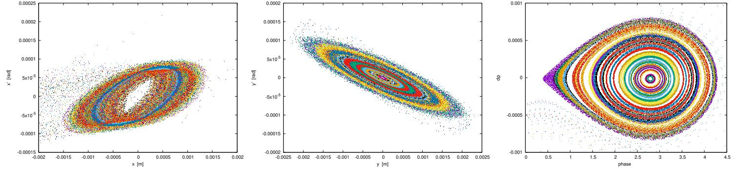
Figure 34: Monitoring: graphs are for 185,000-turn every other 3 turns; 300 particles over the 1,000 tracked (different colors); observation is at 9 o'clock snake.
