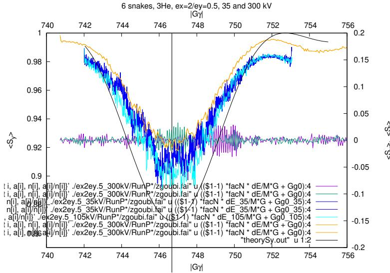
Figure 41: 3He, 6 snakes,  $\epsilon_x/\pi = 2 \mu\text{m}$ ,  $\epsilon_y/\pi = 0.5 \mu\text{m}$ . Turn-by-turn  $\langle S_y \rangle$ ,  $\langle S_l \rangle$  and  $\langle S_x \rangle$  500-particle averages. Blue, orange and cyan: 35 kV (blue), 105 kV (cyan) and 300 kV (orange) cases. Vertical bar: location of the intrinsic resonance  $G_{\gamma_{\text{res}}} = 717 + \nu_y = 746.673$ . Black curve: theoretical envelope (Eq. 2).
