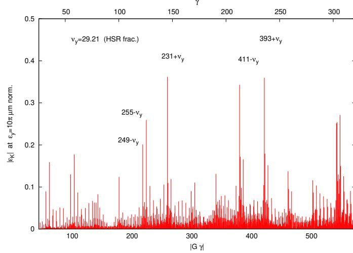
Figure 5: Strength of intrinsic resonances, proton,  $\epsilon_y = 10\pi\mu\text{m}$ , normalized, collision optics, with  $v_y = 29.21$  (optical functions appear to be very similar to the case of nominal tunes of Fig. 2).
