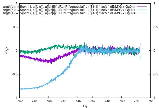
Figure 44: Turn-by-turn  $\langle S_y \rangle$ ,  $\langle S_l \rangle$  and  $\langle S_x \rangle$  1,000 particle averages across  $717+\nu_y$ , helion.
