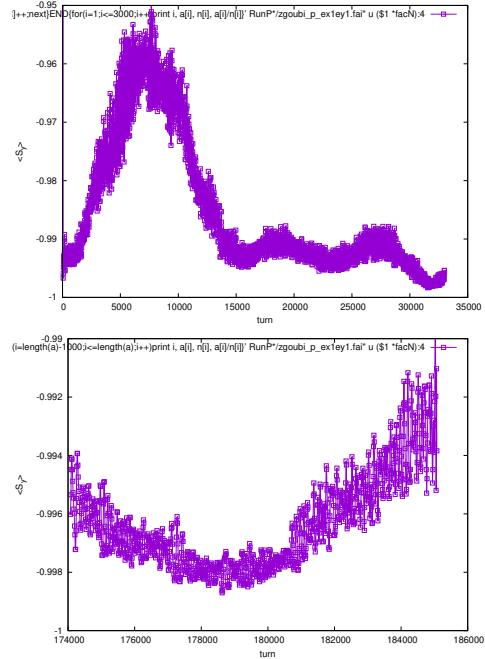
Figure 15: Initial (top) and final (bot.) section of  $\langle S_y \rangle$  (turn) curve of Fig. 14. There is no obvious sign of polarization loss.
