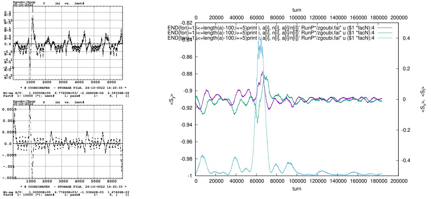
Figure 21: Proton,  $\epsilon_x/\pi = 2 \mu\text{m}$ ,  $\epsilon_y/\pi = 0.5 \mu\text{m}$ , case of 0.302 mm rms vertical defect orbit. Just 1 seed. Left: x orbit, quasi-zero (top) and y orbit, 0.302 mm rms (bottom), 5 turns superposed here, as a sanity check. Right: turn-by-turn  $\langle S_y \rangle$ ,  $\langle S_x \rangle$  1,000-particle averages.
