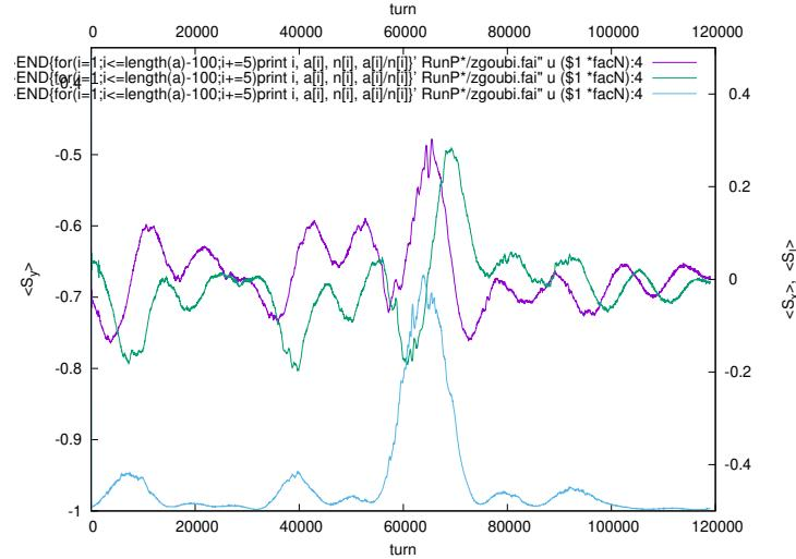
Figure 16: Proton,  $\epsilon_x/\pi = \epsilon_y/\pi = 1 \mu\text{m}$ , case of 0.61 mm rms vertical defect orbit. Just 1 seed. Turn-by-turn  $\langle S_y \rangle$  (left axis), and  $\langle S_l \rangle \langle S_x \rangle$  (right axis) 1,000-particle averages. Difference between upstream and downstream  $\min(\langle S_y \rangle)$  is marginal.
