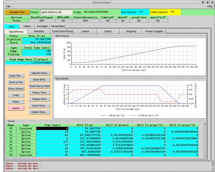
Actual operation uses peak RF voltage of, e.g. in Run 22, 33 kV to 35 kV, for instance  $B\rho\text{-dot}=2$  in Yellow, 4 in Blue, picture above.
