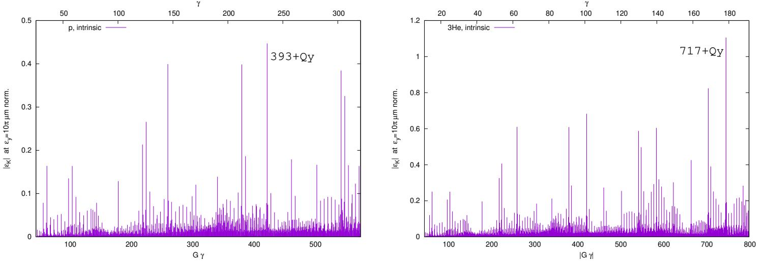
Figure 3: Strength of intrinsic resonances, collision optics, case  $\epsilon_y = 10\pi\mu\text{m}$ , normalized. RHIC is set to  $\nu_y = 29.6730$ . Proton, left graph: the strongest resonance upstream of the 275 GeV EIC as well as RHIC 255 GeV top energy is at  $G\gamma = 393 + \nu_y$ ,  $\epsilon_K = 0.447154$ . Helion, right graph: the strongest resonance upstream of the 170 GeV EIC top energy is at  $|G\gamma| = 717 + \nu_y$ ,  $\epsilon_K = 1.1059$
