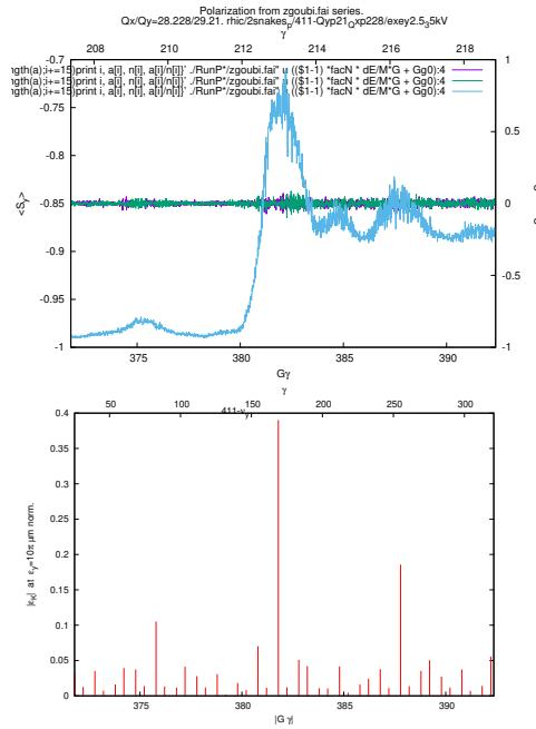
Figure 25: Proton,  $\epsilon_x/\pi = \epsilon_y/\pi = 2.5 \mu\text{m}$ , xing 411-29.21,  $\dot{\gamma} \approx 1/\text{s}$  ( $\hat{V} = 35 \text{kV}$ ). Bottom plot: corresponding resonance spectrum interval from Fig. 5.
