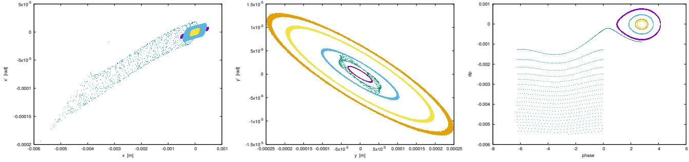
Figure 13: Monitoring: 185,000-turn phase spaces, a few particles (different colors), observation is at 9 o'clock snake. Incidentally, a particle is beyond momentum acceptance here.
