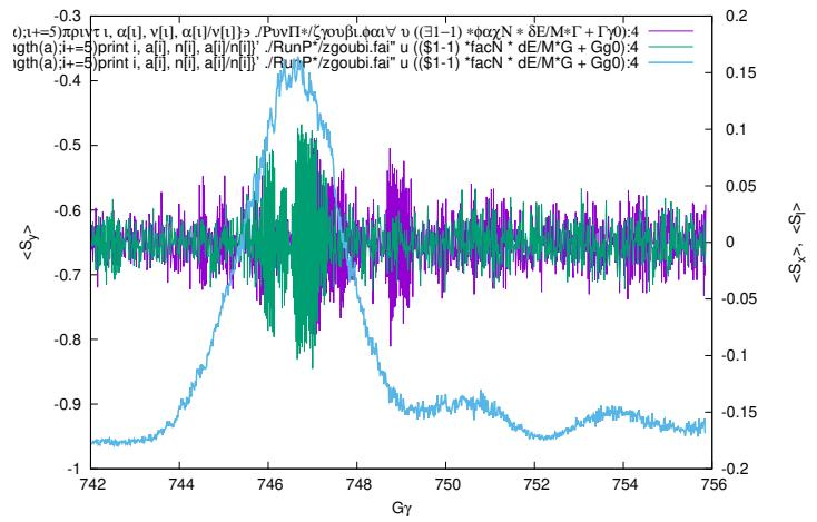
Figure 45: Turn-by-turn  $\langle S_y \rangle$ ,  $\langle S_l \rangle$  and  $\langle S_x \rangle$  1,000 particle averages across 717+ $\nu_y$ , helion.
