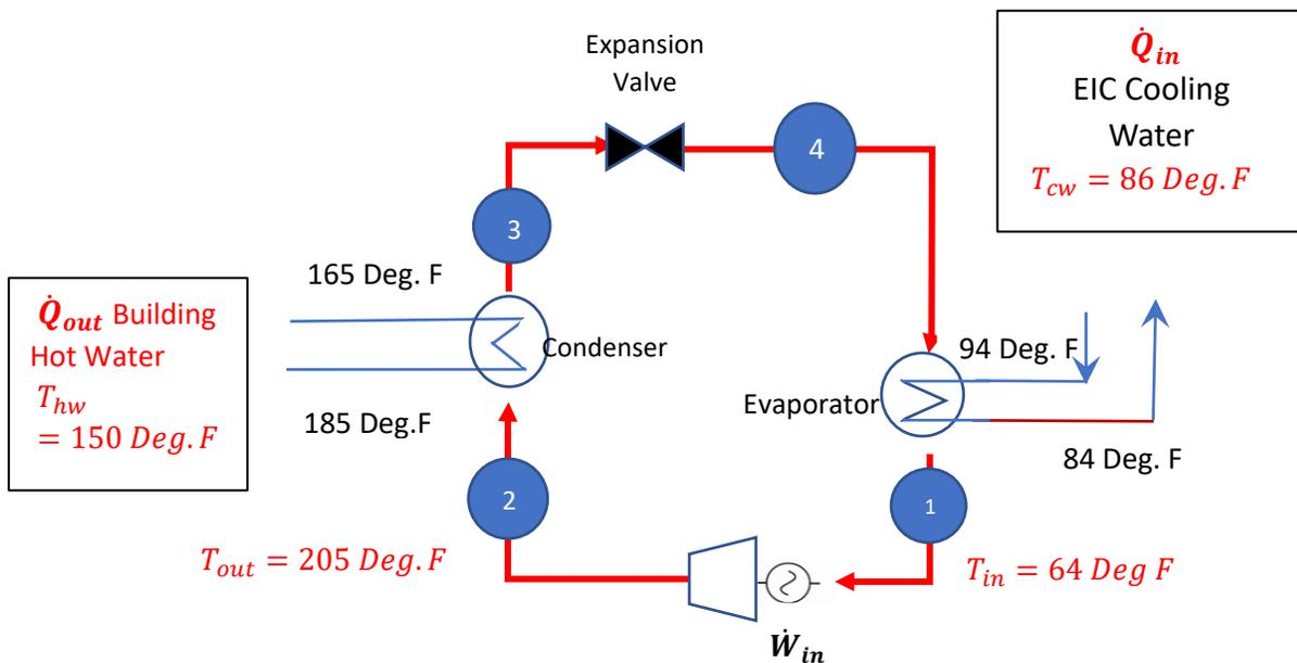
Figure 6 Heat Pump Schematic with Process Conditions
