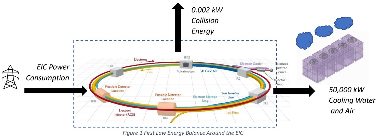
This technical note is prepared to conceptually demonstrate that feasible options exist to recover the low-temperature energy from the EIC cooling water systems.
