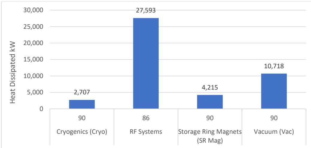
Figure 2 Large cooling water heat loads for EIC
