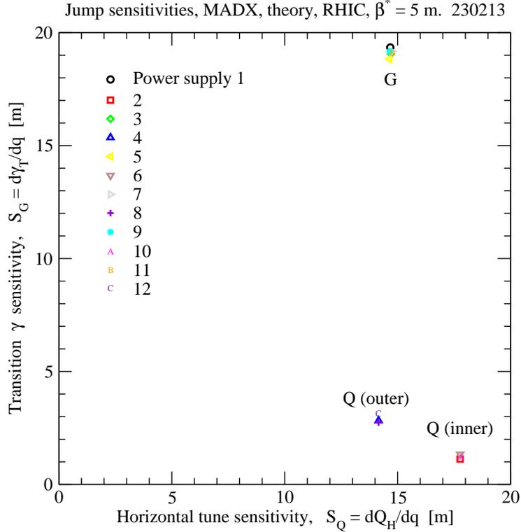
Figure 3: Sensitivities  $S_G$  and  $S_Q$  for the RHIC Yellow jump quad power supplies, with  $\beta^* = 5$  m at each IP. All 6  $S_G$  values are similar, while the  $S_Q$  values are somewhat different in the inner and outer arcs.
