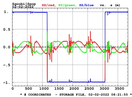
Figure 97: Vertical component of spin  $\vec{n}_0$  around RHIC Yellow. Case of a spin defect (some arbitrary spin rotation, located at IP8 in the present case), rotators off.
