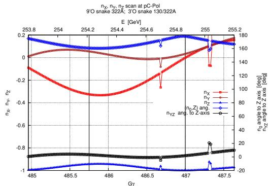
Figure 77: Spin  $\vec{n}_0$  components vs.  $G\gamma$  in 255 GeV region, at pC-polarimeter.  $\vec{n}_{YZ}$  denotes the projection of  $\vec{n}_0$  in the (Y,Z) plane.
