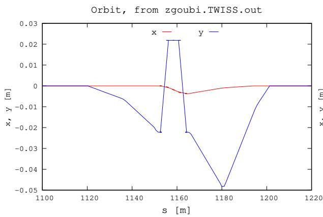
Figure 20: Closed orbit bump in 9 o'clock snake region (the 10.4 m snake extends around  $s \approx 1160$  m), case of 300 Amp in coils 1-4, an excerpt from Fig. 19. Note that the peak vertical excursion (-5 cm) can be reduced (below 3 cm) by introducing a positive incidence of the orbit at entrance to the snake ( $s = 1151$  m)
