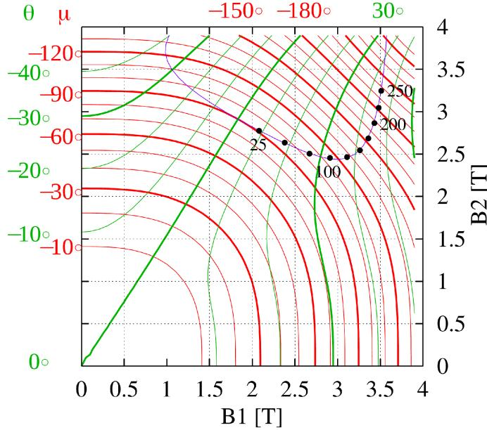
Figure 101: From Ref. [4]. Field dependence of the spin precession angle ( $\mu$ ) and precession axis angle to the radial axis ( $\theta$ ; the precession axis is in the transverse plane).  $B_1$  and  $B_2$  are field values in respectively the outer and inner pair of coils. 25 to 250 GeV set points (black dots) compare well with present simulation outcomes.
