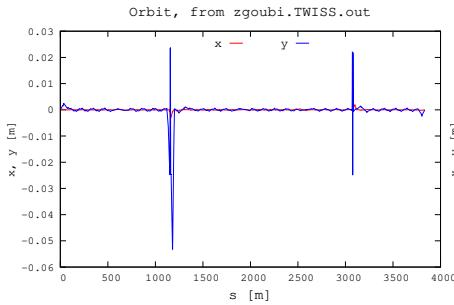
Figure 43: H and V RHIC orbits. The vertical excursion inside 9o'clock snake (at  $s \approx 1200$  m) is 24 mm, the 52 mm excursion observed here is *outside, downstream of the snake*, result of a simplistic bump closure.
