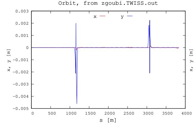
Figure 47: Orbits with snake bumps. IP bump zero-ed.
