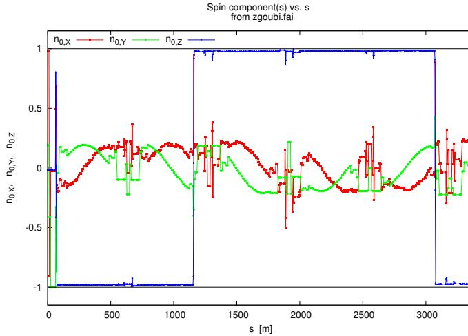
Figure 94: Spin  $\vec{n}_0$  components around yellow, 255.200 GeV. Longitudinal ( $n_{0,X} = 1$ ) in STAR region ( $s=0$ ), mostly vertical elsewhere ( $n_{0,Z} = 1$ ). With the present settings (complete snake and nominal rotator settings) the spin tilt from longitudinal at STAR is 11 deg, it is 14.3 deg at pC-polarimeter. The spin component spikes seen on this graph occur at the vertical separation bumps at IPs
