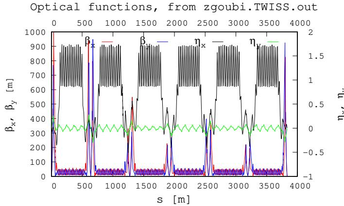
Figure 90: Optics with snake and STAR rotator field maps as part of the Yellow-CW model. Fractional tunes  $\nu_Y = 0.69094$ ,  $\nu_Z = 0.68484$ . Chromaticities  $\xi_Y = 4.7/\xi_Z = 5.2$ . IP6  $\beta_{Y,Z}^* = 1.38$ , 1.46 m.
