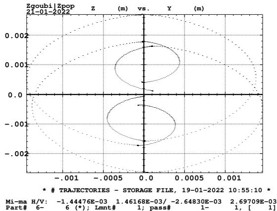
Figure 88: Transverse projection of helical trajectories in snakes.
