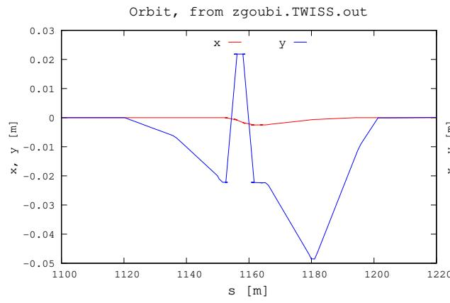
Figure 33: Orbit in 1&3 coil 9 o'clock snake 320 Amp, an excerpt from Fig. 32. Note that the peak vertical excursion (0.05 m) can be reduced (to  $\lesssim 3$  cm) provided a positive orbit incidence at snake entrance
