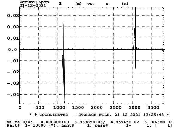
Figure 38: Typical vertical closed orbit around RHIC Blue, prior to fitting
