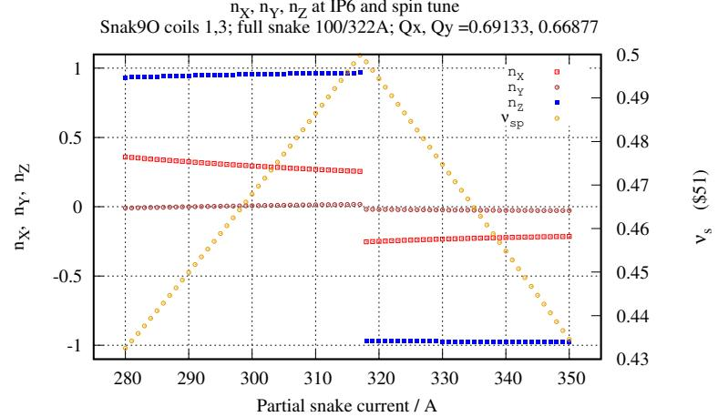
Figure 36: A scan of the components of RHIC Blue spin eigenvector  $\vec{n}_0$ (IP6), and spin tune, versus current in coils 1 & 3 of 9 o'clock snake. Current is varied from 280 to 350 A. Higher current yields  $\vec{n}_0$ (IP6) closer to vertical
