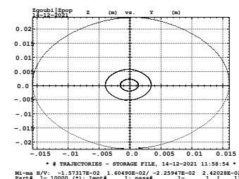
Figure 14: YZ projection of orbits at 255, 100 and 23 GeV.
