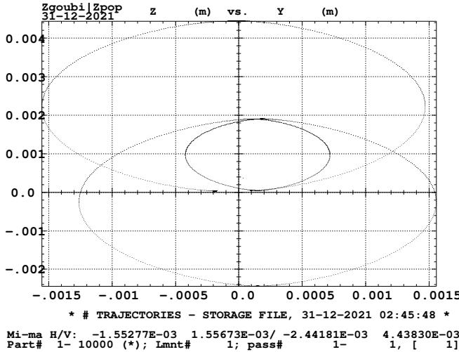
Figure 69: Y-Z projection of helical orbits in (upper one) 9 o'clock/322A and in (lower) 3 o'clock/130A/322A snakes. 255 GeV.
