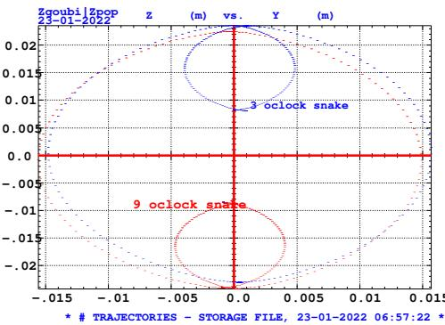
Figure 84: Transverse projection of helical trajectories in snakes, injection.
