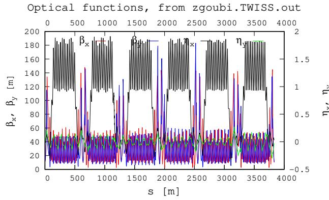
Figure 80: RHIC Yellow injection optics with snake field maps only. Coil currents 100/322 Amp. Fractional tunes  $\nu_Y = 0.7032/\nu_Z = 0.6837$ . Chromaticities  $\xi_Y \approx 2/\xi_Z \approx 11$ . IP6  $\beta_{Y,Z}^* = 10.0/9.9$  m.
