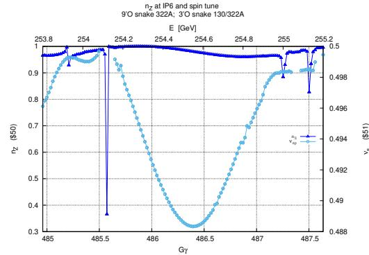
Figure 79: Spin  $n_Z$  component at STAR, and spin tune.
