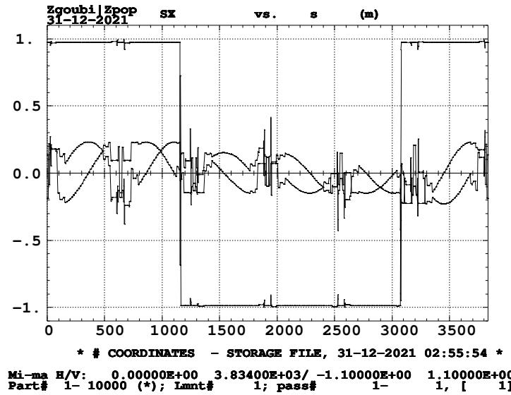
Figure 73: Spin  $\vec{n}_0$  components around RHIC Blue. 255 GeV.
