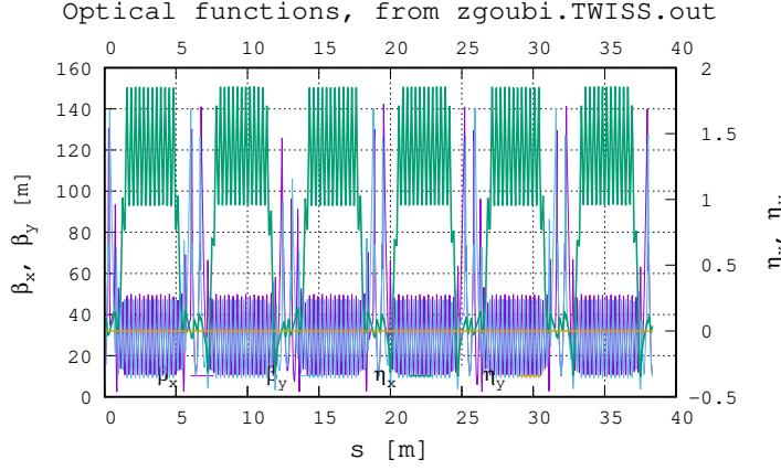
Figure 31: Optics at 320 A in coils 1 & 3. Fractional tunes  $\nu_Y = 0.69133/\nu_Z = 0.66877$ . Chromaticities  $\xi_Y = -12.759/\xi_Z = 3.42815$ . IP6 and IP8  $\beta_{Y,Z}^* = 1.5$  m.
