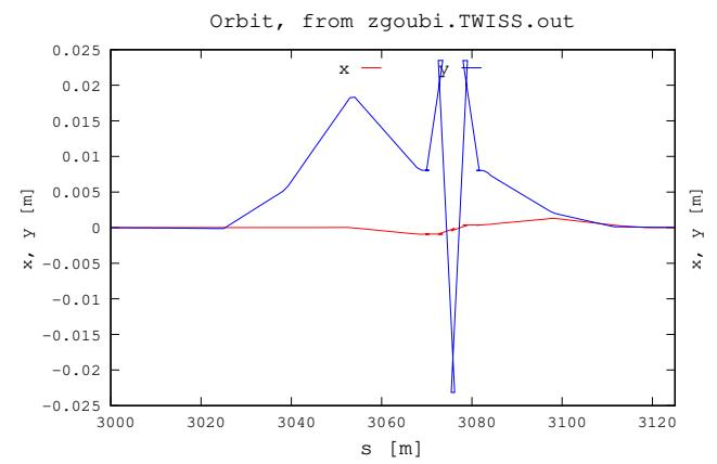
Figure 34: Orbit in complete 3 o'clock snake, 100/322Amp coil currents, an excerpt from Fig. 32.
