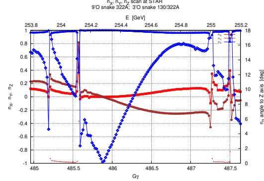
Figure 78: Spin  $\vec{n}_0$  components at STAR, and spin angle to Z (vertical) axis.
