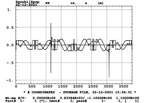
Figure 56: horizontal components of spin eigenvector around RHIC Blue
