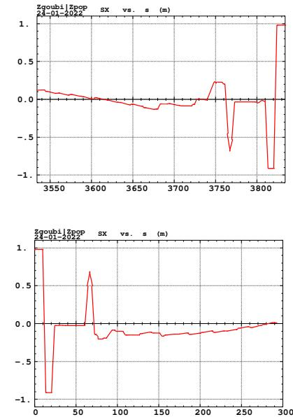
Figure 95: Details of longitudinal spin  $\vec{n}_0$  component in STAR region in yellow, 255.200 GeV.
