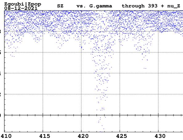
Figure 25: At IP6, tracking  $S_Z(G\gamma)$  across  $393 + \nu_Z$ , single particle on  $\epsilon_y = 2.5 \pi \mu\text{m}$  normalized invariant. Spin starts vertical, obviously away from  $\vec{n}_0$ , however final oscillation of  $\vec{S}$  has similar amplitude, indicating absence of depolarization. See Figs. 26-30 for more
