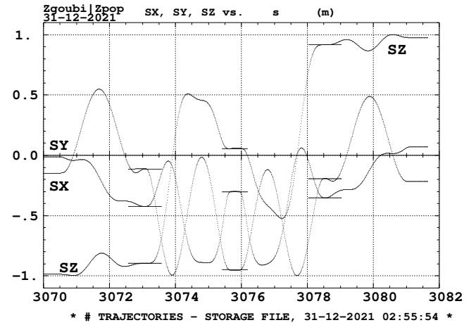
Figure 72: Spin  $\vec{n}_0$  components across 3 o'clock snake. 255 GeV.
