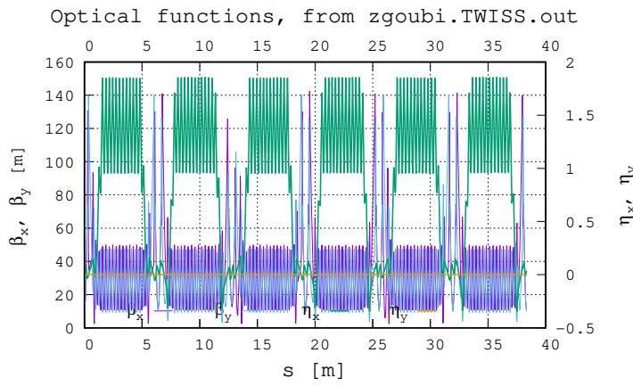
Figure 18: Optics with field maps, 300 A in coils 1 & 4. Fractional tunes  $\nu_Y = 0.69068/\nu_Z = 0.66596$ . Chromaticities re-tuned to  $\xi_Y = 1.9265/\xi_Z = 7.2696$ . IP6 and IP8  $\beta_{Y,Z}^* = 1.5$  m.
