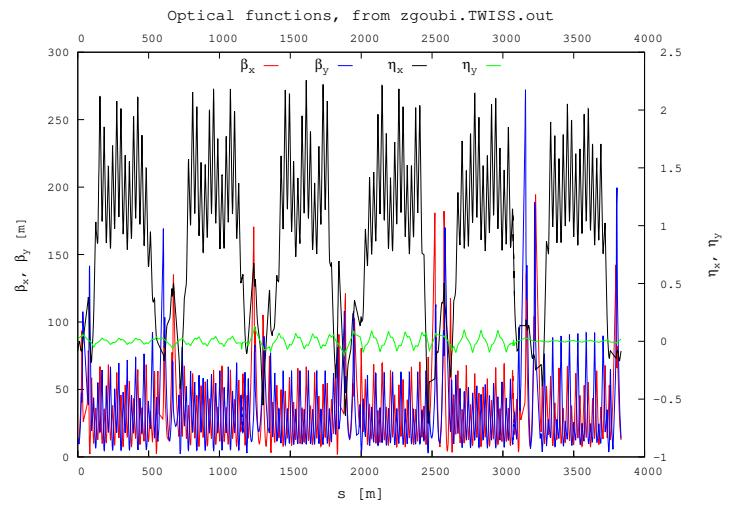
Figure 59: Blue optics at injection from Zgoubi model, brute from MADX translation and including snake OPERA field maps. Current in 9 o'clock snake is 320 A (coils 1 & 3), currents in 3 o'clock snake are 130/322 A.
