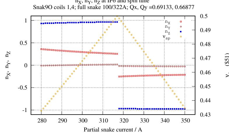
Figure 23: A scan of the components of RHIC Blue spin eigenvector  $\vec{n}_0(IP6)$ , and spin tune, versus current in coils 1 & 4 of 9 o'clock snake. Current is varied from 280 to 350 A. Higher current yields  $\vec{n}_0(IP6)$  closer to vertical
