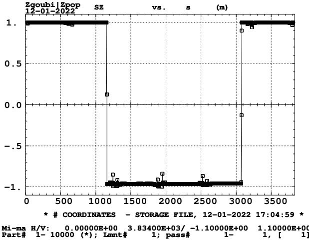
Figure 74: Vertical spin component  $n_Z$  around RHIC Blue, at  $G\gamma = 485.75$  (254.21 GeV/c).  $n_Z = 0.99802$  at STAR. Note: as expected,  $\vec{n}_0$  is seen to move away from vertical at IP separation bumps rise and fall
