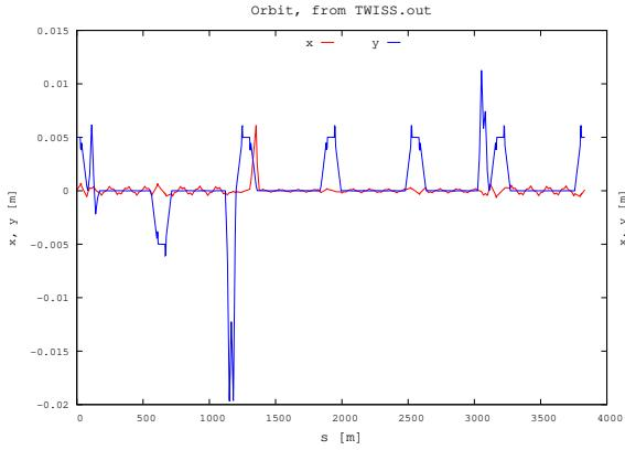
Figure 60: Closed orbits with snake bumps, from MADX.
