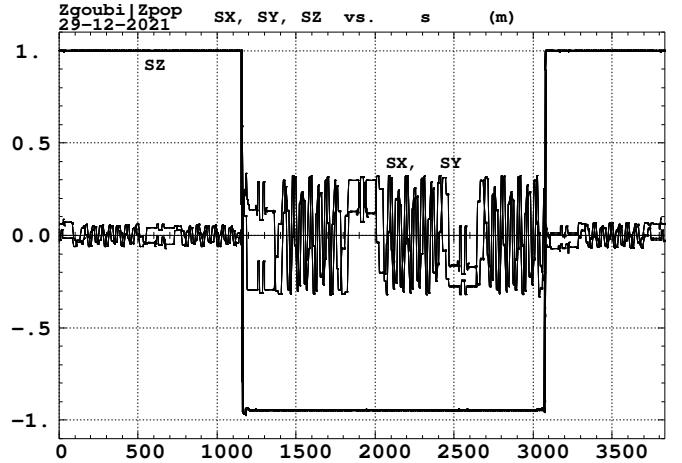
Figure 64: Components of the periodic spin vector around RHIC. Origin s=0 is at IP6.
