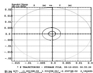
Figure 6: YZ projection of orbits at 255, 100 and 23 GeV.
