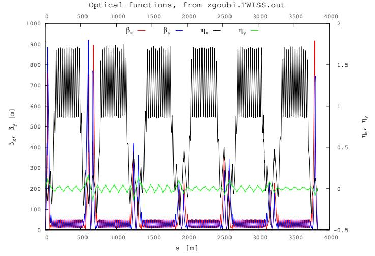
Figure 66: Blue optics at store energy, from Zgoubi model, which includes snake OPERA field maps. Current in 9 o'clock snake is 320 A (coils 1 & 3), currents in 3 o'clock snake are 130/322 A.
