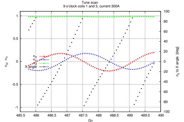
Figure 51: A scan of spin eigenvector components vs. energy, around RHIC Blue, 255 GeV
