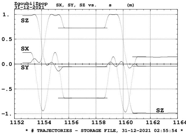
Figure 71: Spin  $\vec{n}_0$  components across 9 o'clock snake. 255 GeV.
