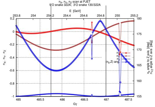
Figure 76: Spin  $\vec{n}_0$  components vs.  $G\gamma$  in 255 GeV region, at H-Jet.
