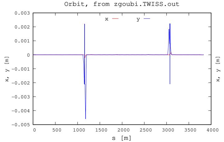
Figure 53: Orbits with snake bumps. IP bumps zero-ed.
