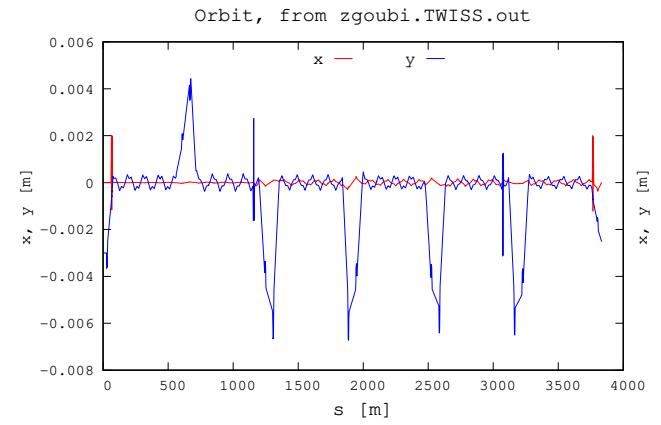
Figure 91: Orbits with snake and STAR rotator field maps. IP bumps suffer a little and a fraction of mm closed orbit is excited, however the residual orbit is considered of marginal effect regarding the goals of the present study, and left as it comes
