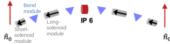
Figure 2: The spin rotators are composed of short- and long-solenoid modules, as well as bend modules, to rotate the spin from vertical in the arcs to longitudinal at the IP and back to vertical on the other side.
