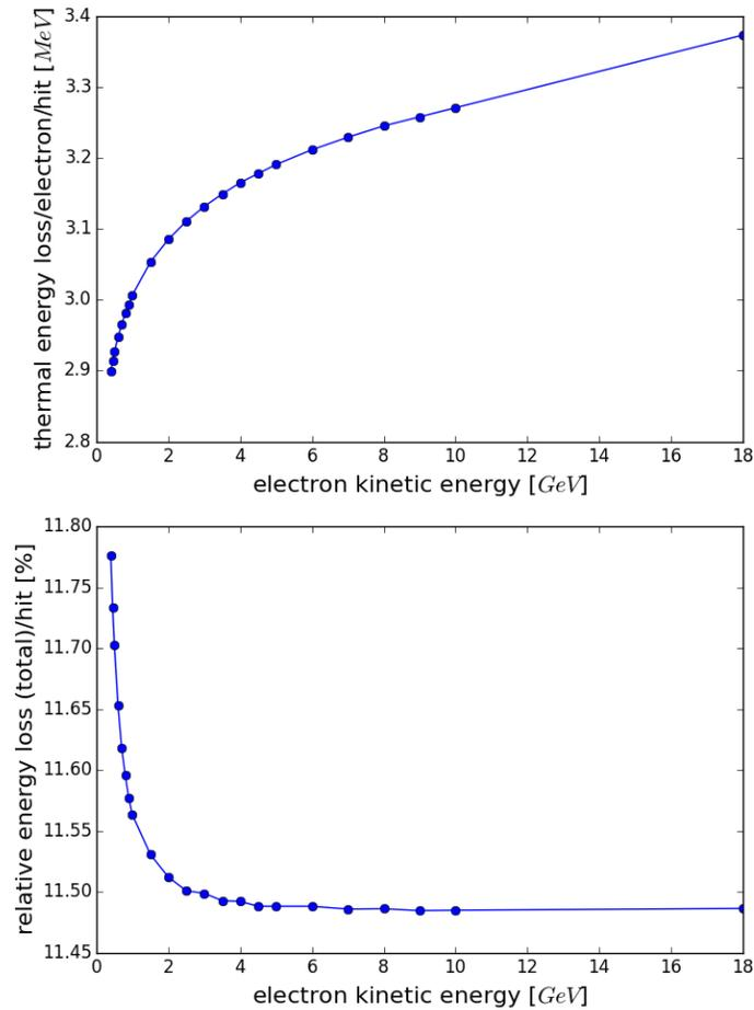
Figure 3: Electrons energy loss on a single hit.
