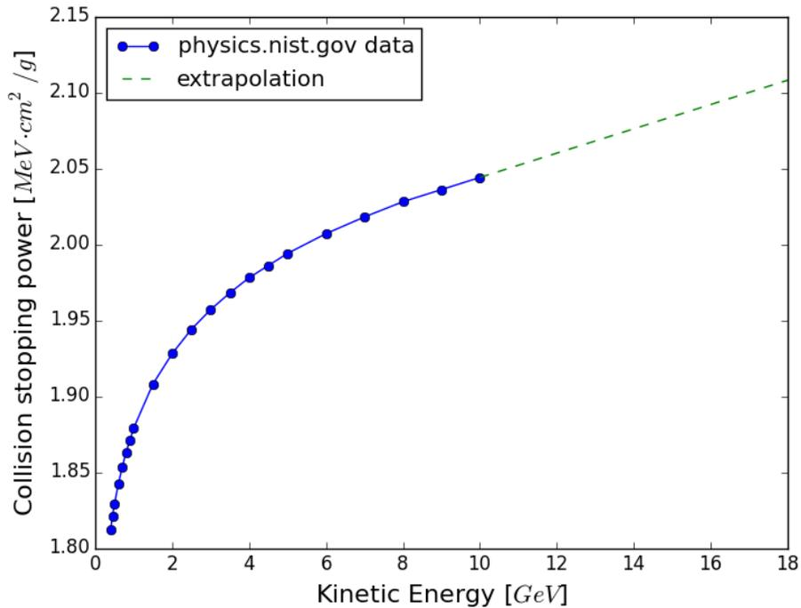
Figure 2: Stainless steel collision stopping power for electrons.
