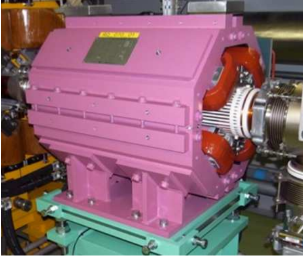
FIG. 27: The J-PARC ripple correction quadrupole.
