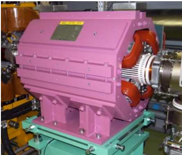
FIG. 27: The J-PARC ripple correction quadrupole.
