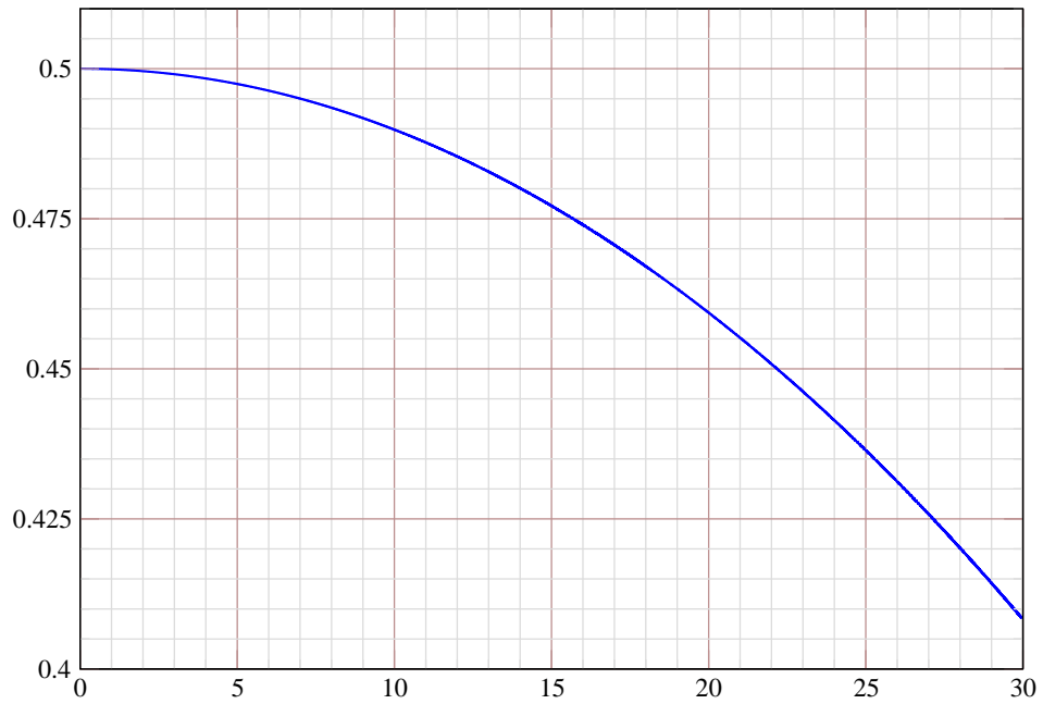
Figure 30: V_2/V_1 obtained from (78), (79), and (80) as a function of \phi_1 for Flattened Bucket Option II. The horizontal axis is \phi_1 marked in degrees.
