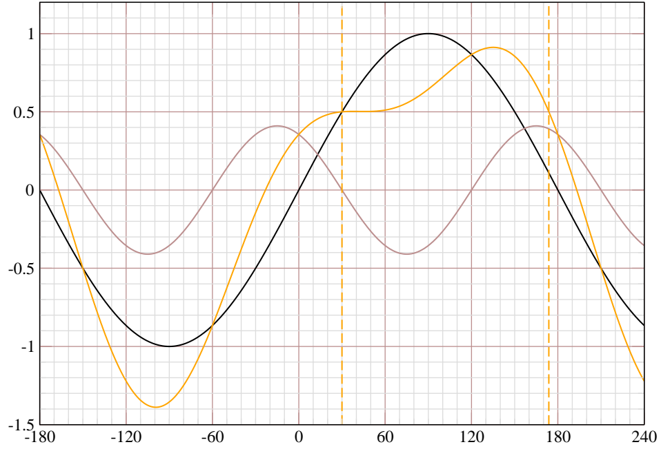
Figure 16: Normalized harmonic 1 and 2 voltages and their sum \mathcal{V}(\psi) = \sin \psi - (V_2/V_1) \sin(2\psi - 2\phi_s) for double harmonic acceleration in Booster. These are the black, brown, and orange curves, respectively. The stable and unstable synchronous phases are marked by the dashed vertical lines at 30 and 173.745 degrees respectively. Here we have used Flattened Bucket Option I with \phi_s = \phi_1 = 30^\circ , \psi_0 = 30^\circ , and V_2/V_1 = 0.41 , just as in Figures 1 and 2 . Note that the harmonic 2 voltage (brown curve) goes from positive to negative and the sum of the voltages is flattened as the phase \psi passes through the stable synchronous phase.
