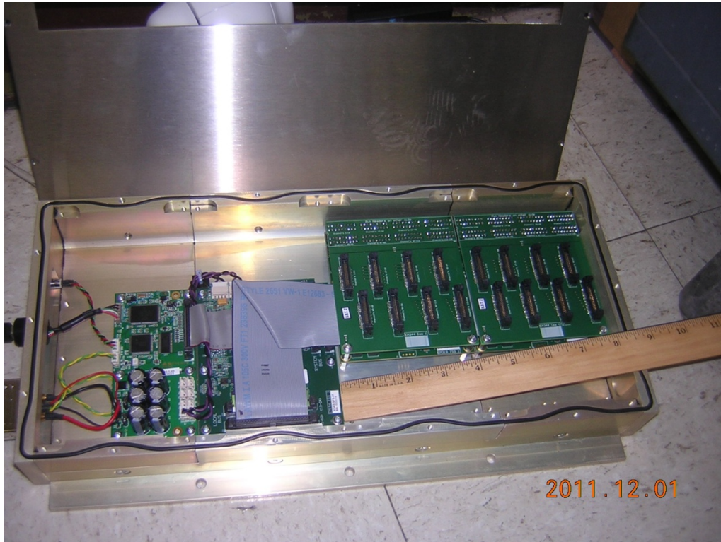
Figure 2: The V3 system is more densely packed and compact than the HE system. Notice that the boxes of the two systems are the same size.
