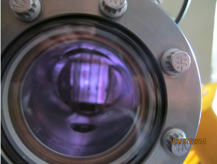
Figure 1: Glow discharge during Argon sputter cleaning of SEC (2 foils only) with positive high voltage applied.
