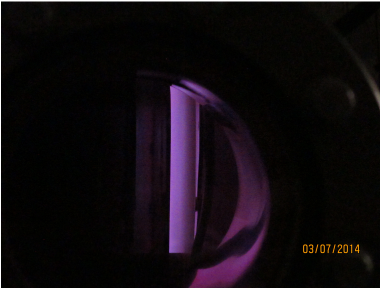
Figure 2: Glow discharge with negative HV.
