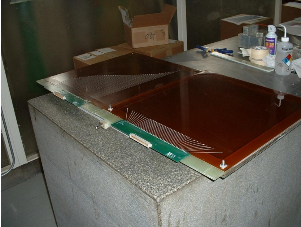
Figure 15: Back side of the 302 ion chamber, showing connections to the readout PC board.
