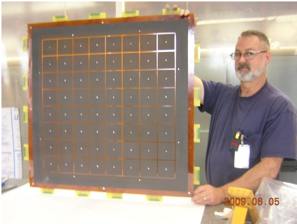
Figure 10: The 8x8 pixel plane. Each pixel is 8 cm square.
