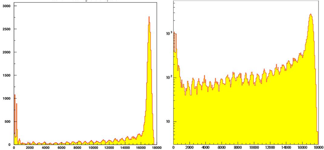
Figure 1: Scintillator response to a 1000 MeV/n Iron beam fragmenting in 4.86 g/cm<sup>2</sup> Aluminum target. Horizontal axis is in ADC counts. The vertical scale is linear/logarithmic on the left/right panel.
