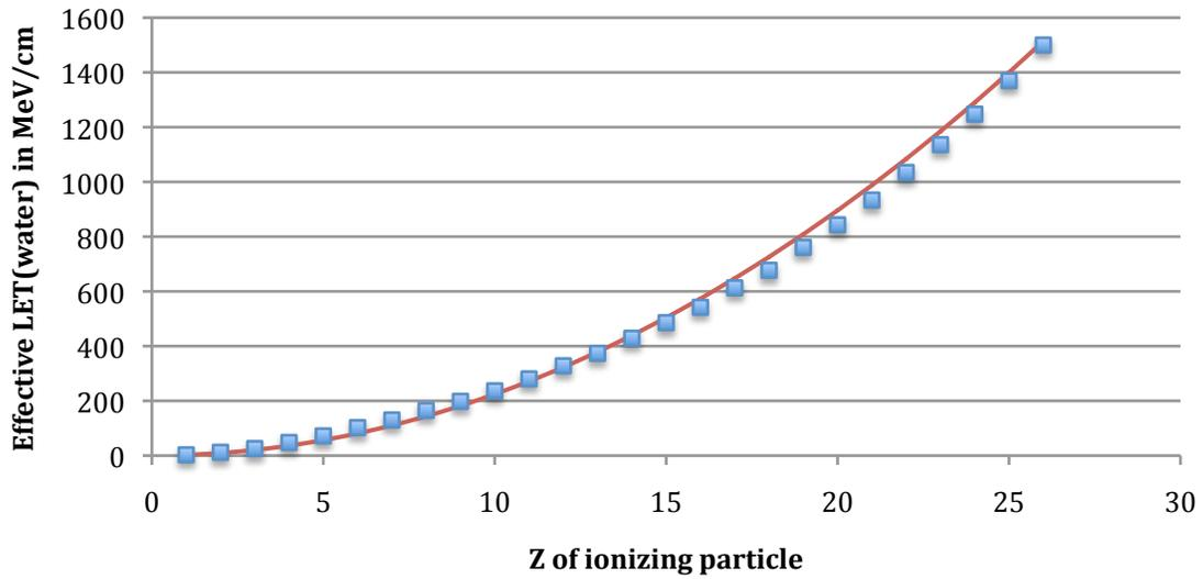
Figure 4: Comparison of the expected LET(water) for a 1000 MeV/n beam of atomic number  $Z$ , and the measured energy response after calibration. The expected energy response, scaling with  $Z^2$ , is the red line, while the data points show the measurement.
