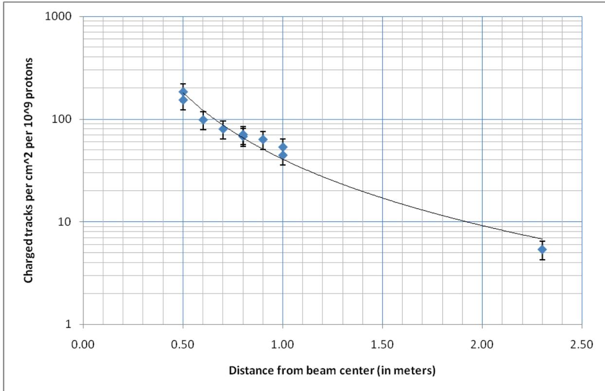
Figure 6: Charged particle flux as a function of the distance from beam center in meters. The flux is in units of charged particles per square cm per  $10^9$  incident 200 MeV protons. The fit is a power law in R, the distance from beam center, using the power -2.15.
