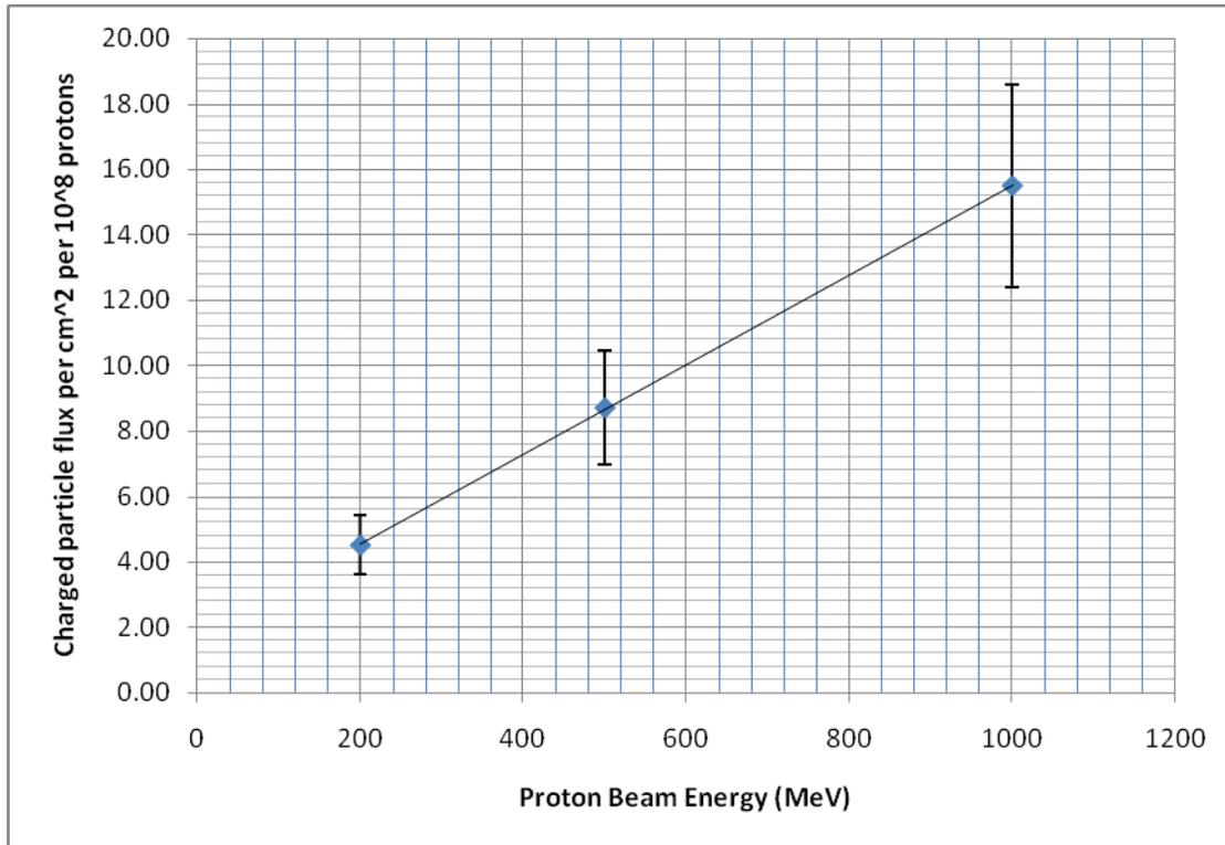
Figure 7: Charged particle rate per square cm per  $10^8$  incident protons as a function of the proton beam kinetic energy, in MeV. These rates were measured at a location that was 0.9 meters away from beam center transversely, and 1.9 meters downstream of the Booster vacuum window.
