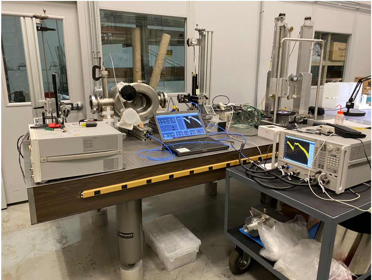
Figure 1: Stretched wire pulled through the DQW crab cavity beam pipe.
