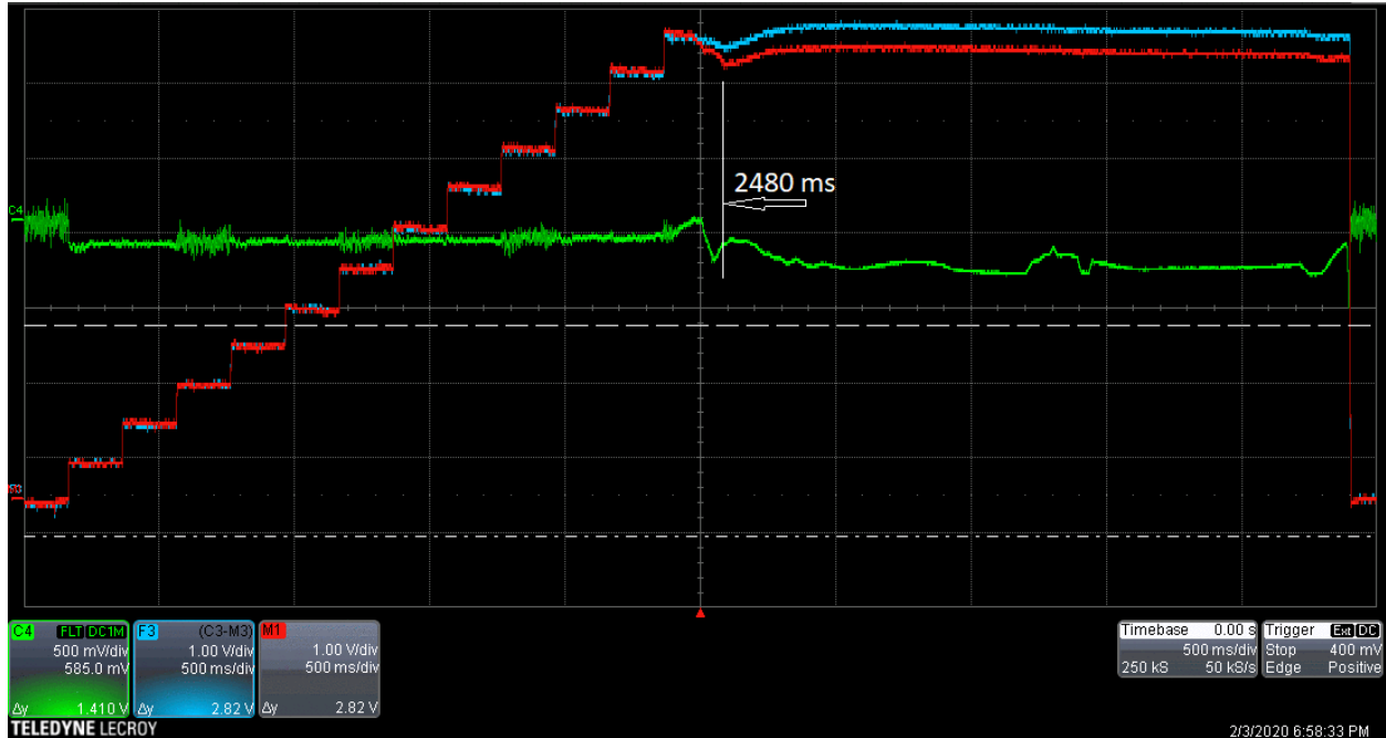
Figure 23: The AGS normalized transformer on the 24-16-8 merge 4.59 GeV cycle with EBIS Au (setup 7 in Table I) with octupoles on (blue) and off (red). The trigger is At0+2400 ms. The magnet ramp begins at 2480 ms. AGS Late is about 6e9 . 67
