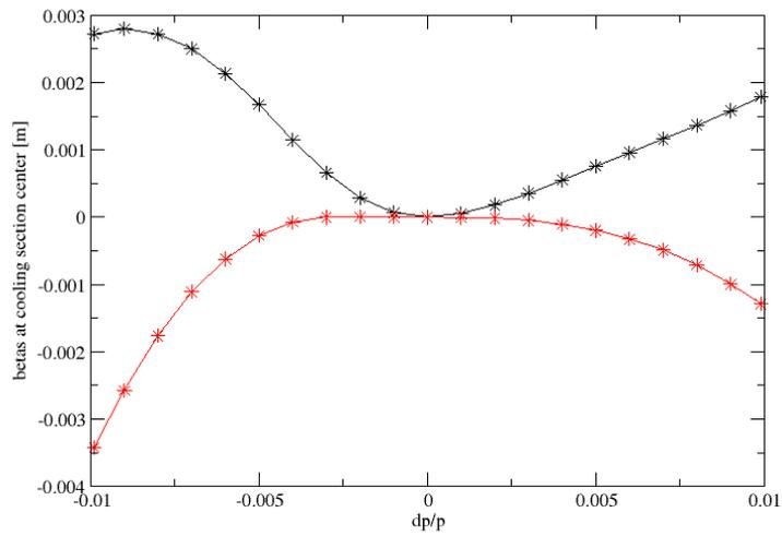
Fig. 12: Orbit in the center of the cooling section as function of constant energy deviation. Because of the ring symmetry the slope of the orbit is zero at this location.
