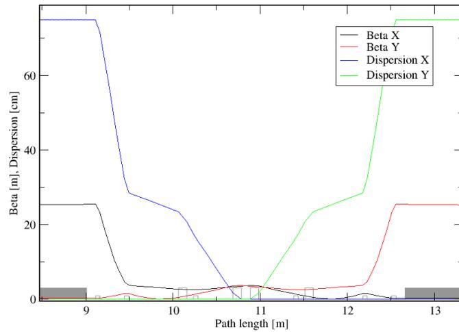
Fig. 2: Twiss functions in the transition between wigglers
