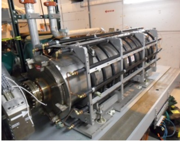
FIG. 20. Example of the LEReC high-power beam dump.
