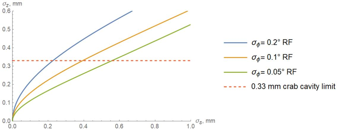
Figure 5: Beam arrival position jitter vs. integrated feedback sensor noise for several rms values of RF phase noise,  $\sigma_\phi$ . Bandwidth of  $[0.5 \ 1.5]\omega_s$  is assumed for both the RF and sensor noise.
