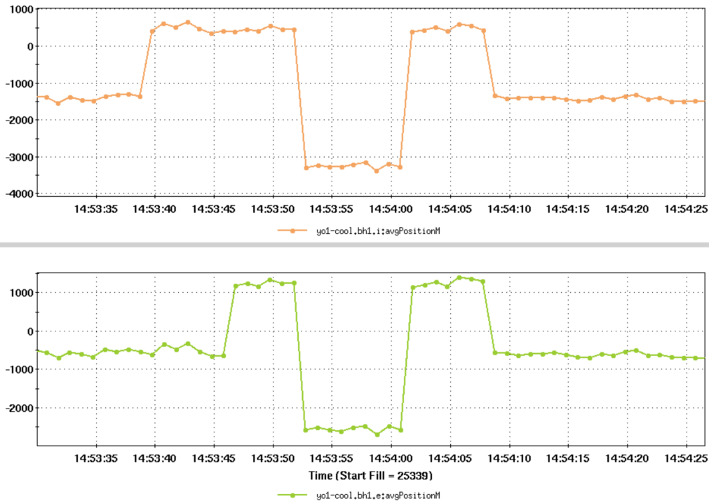
Figure 2: The test of auto-switching script. Initially the auto-switching is off. At 14:53:40 an artificial imbalance is introduced to the channels of 9 MHz BPM. At 14:53:47 the imbalance is introduced to the 704 MHz BPM. At 14:53:52 the channels are manually switched, at 14:54:02 the channels are manually switched back. At 14:54:09 the auto-switching is turned on. The electron beam was in the 76 kHz mode with 5 macro-bunches during this test.
