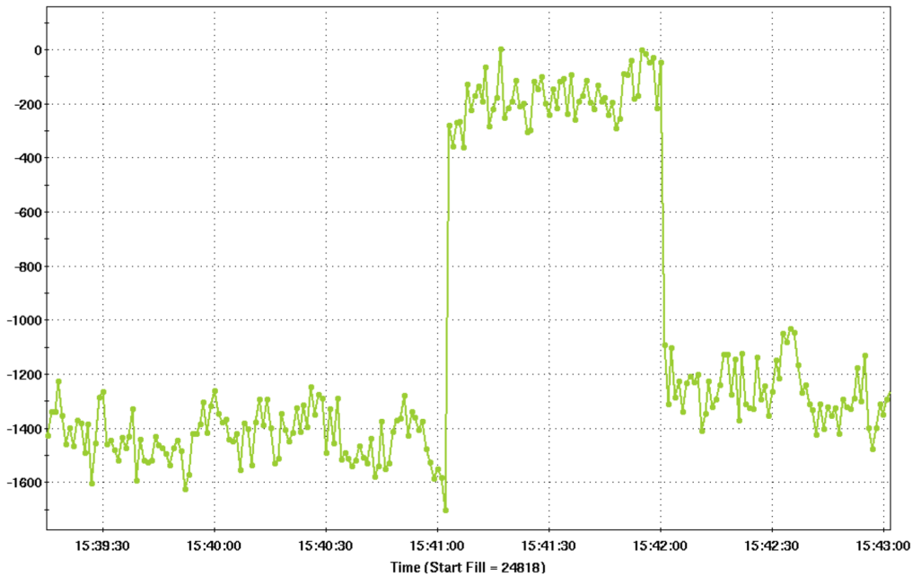
Figure 1: One of the CS BPMs showing a large change in position measurement when the channels are switched. The electron beam was in the CW mode during this test.
