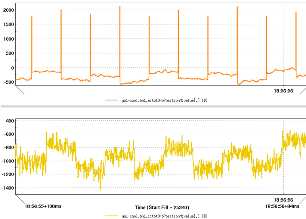
Figure 5: The switching transients were observed on turn-by-turn data from 704 MHz BPM board (upper plot). No transient effect was seen from 9 MHz board (lower plot).
