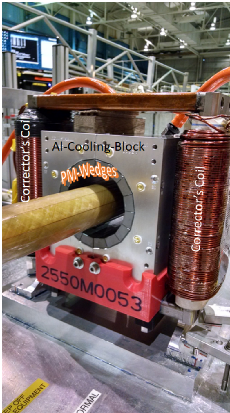
Figure 5: A picture of the quadrupole permanent magnet wedges surrounded by the Al cooling block. The coils of the dipole corrector magnet are also shown.
