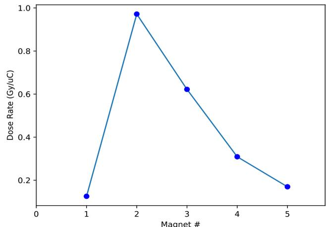
Figure 5: Model I Average Dose Rate per Magnet
