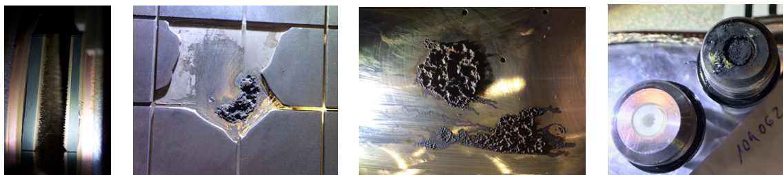
Figure 3.2.7: Images from damaged circulators. The panels show ferrites on a 5 kW circulator contaminated with plastic insulator material, damage to the load plates on a 10 kW and a 5 kW circulator respectively. The rightmost panel shows a damaged screw and its replacement.
