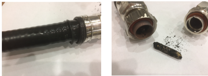
Figure 3.2.4: Damage to an internal cable connecting a single module to the power combiner in a 5 kW SSA which led to the failure of the associated power module.
