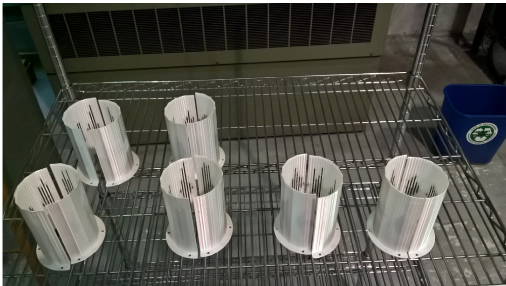
Figure 0.9.14: The 3D printer support plastic folders for the magnetic field corrections with iron wires.
