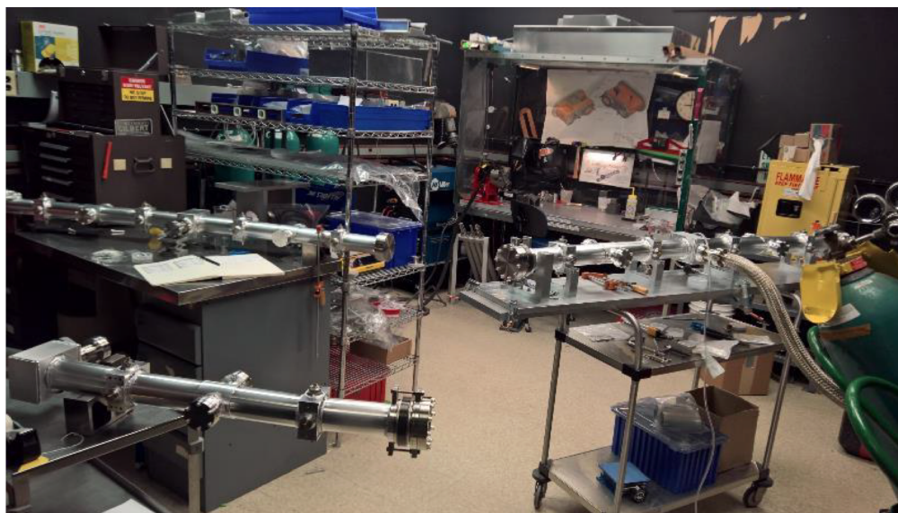
Figure 0.7.1: Vacuum system development for the S1 splitter line.
