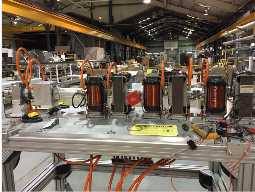
Figure 0.5.2: The photograph of the last stage in production and assembly of the first fixed field magnet girder.
