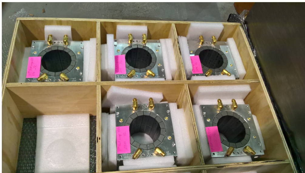
Figure 0.9.7: Due to a very strong magnetic field the assembled magnets needed to be safely packed in the boxes, separate from each other, for air transport.
