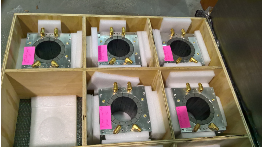
Figure 0.9.7: Due to a very strong magnetic field the assembled magnets needed to be safely packed in the boxes, separate from each other, for air transport.
