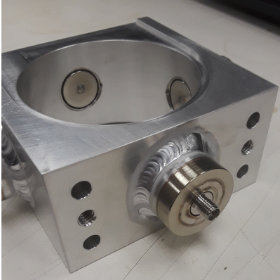
Fig 2. FFA loop BPM button chambers Button diameter: 20 mm BPM chamber diameter (FFA beam pipe diameter): 2.756 inches (70 mm) Expected horizontal beam variations in FFA: \pm 24 mm
