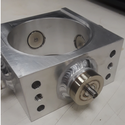
Fig 2. FFA loop BPM button chambers Button diameter: 20 mm BPM chamber diameter (FFA beam pipe diameter): 2.756 inches (70 mm) Expected horizontal beam variations in FFA: +/-24 mm
