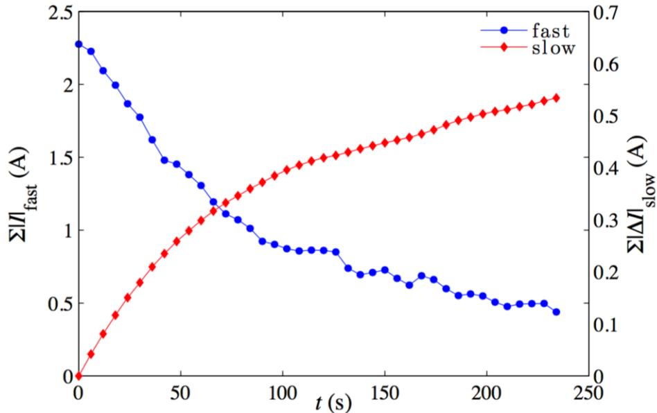
Fig. 2. Sum current of all horizontal fast correctors (blue) and sum current of all horizontal slow correctors (red). The total time is about 4 min.
