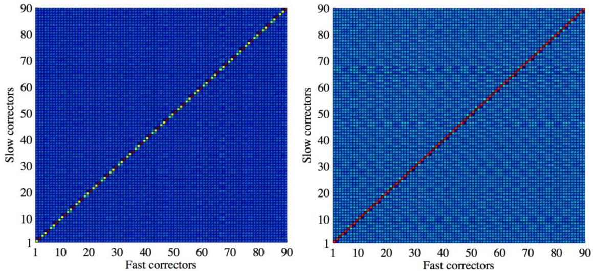
Fig. 1. Modeled fast-to-slow corrector-shifting matrices: horizontal (left) and vertical (right).
