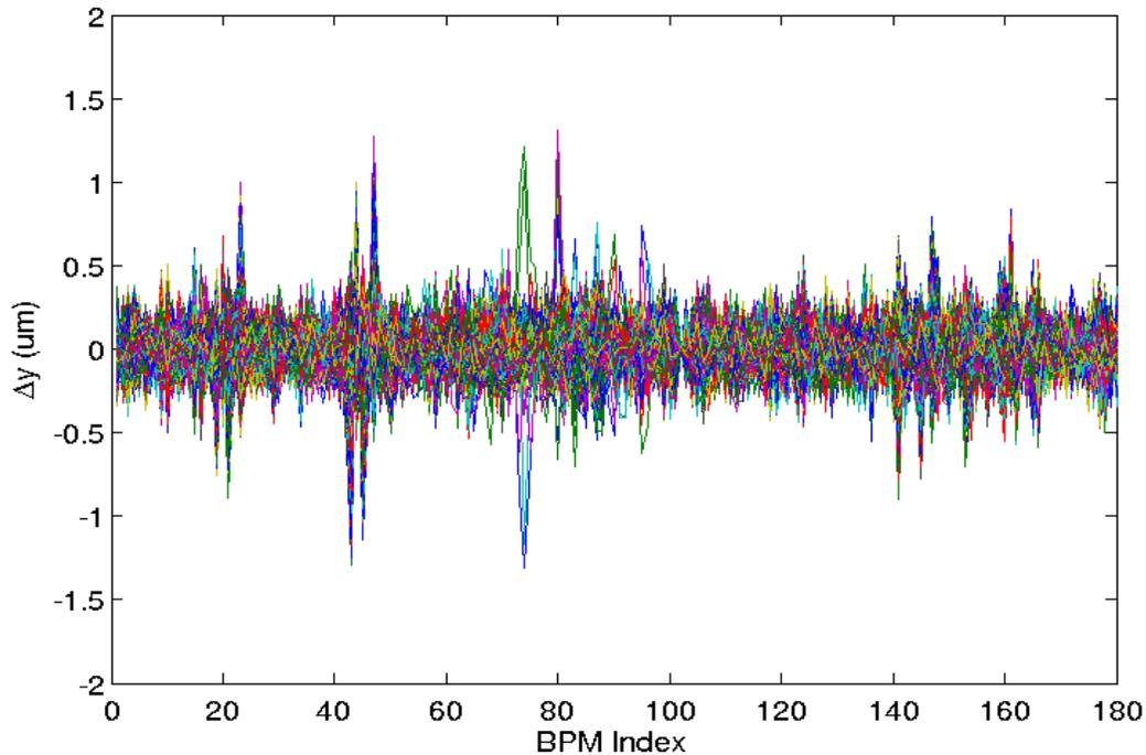
Fig. 5 The vertical orbit deviation measured by all 179 good BPMs during the shifting process.
