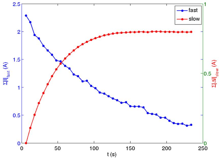
Fig. 4. Sum current of all vertical fast correctors (blue) and sum current of all vertical slow correctors (red). The total time is about 4 min.
