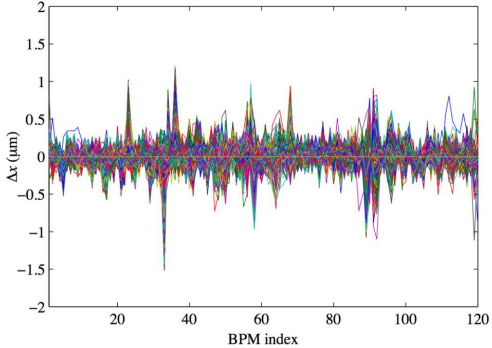
Fig. 3 The horizontal orbit deviation measured by 120 non-dispersive BPMs during the shifting process.
