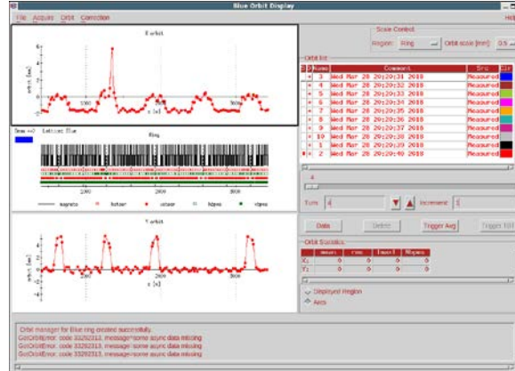
Figure 4: The horizontal orbit shifted inwards by \sim 2 mm in the ring due to expected difference of RHIC dipole transfer function with the new magnet cycle.
