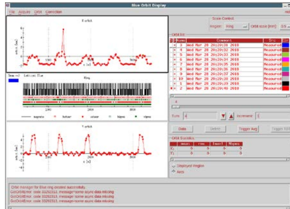
Figure 4: The horizontal orbit shifted inwards by \sim 2 mm in the ring due to expected difference of RHIC dipole transfer function with the new magnet cycle.
