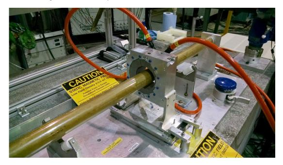
The measurements were conducted with the magnet's water channels connected to a chiller loop run at 85F (the nominal operating temperature for these magnets), so that the temperature coefficient of the permanent magnet material would not give incorrect results.
