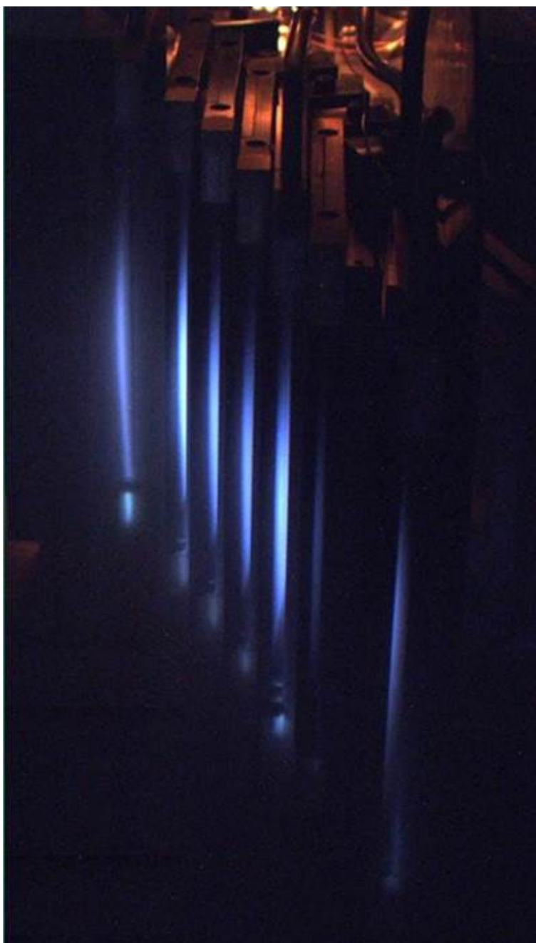
Figure 10: Ruthenium isotope separation at ORNL. Here the blue glow is due to photoemission as the ion beam interacts with background gas in the vacuum chamber. The glow furthest to the right is due to ^{96}\text{Ru} ions. With permission and courtesy of ESIPP at ORNL.
